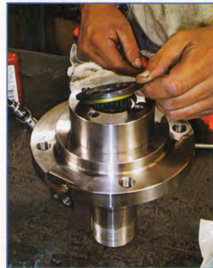
A replaceable seal on the back of the needle-bearing housing allows the bearing to be repacked with grease at normal intervals.
