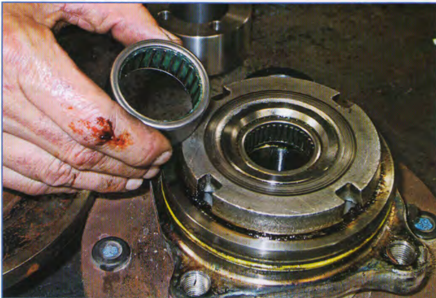
The replacement needle bearings are significantly larger than those in the factory-unit hub.
